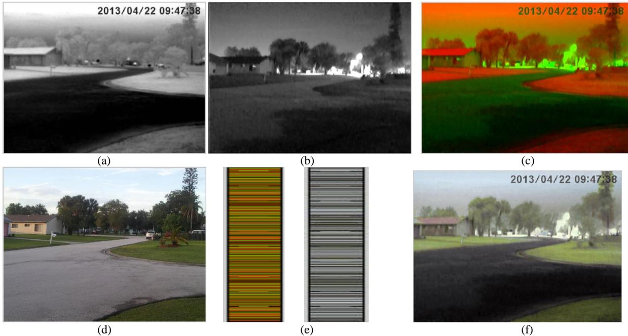
Figure 2 Images of same scene used in example (a) preprocessed IR image (b) preprocessed visible image (c) fused false color image (d) reference image (e) false-color (on left) and derived (on right) colormaps (f) final result.
