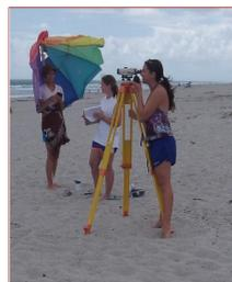
Figure 2A (left): Looking through level and tripod to read the stadia rod and the elevation
