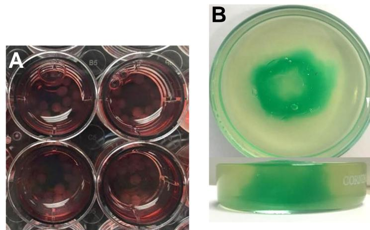
**Figure 2:** A) Cell-containing alginate beads in wells filled with media; B) 3D printed alginate (green) hydrogel printed into petri dish of gelatin support bath for precision test
