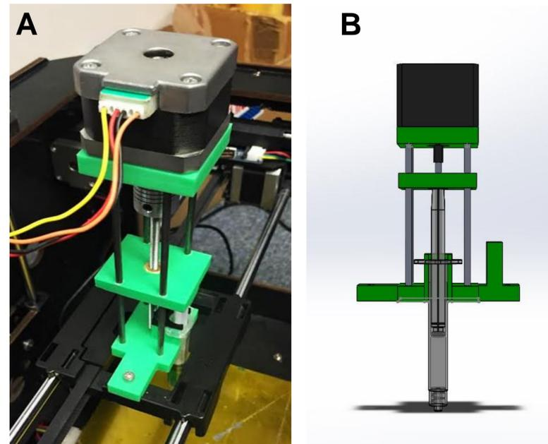
**Figure 1:** A) Overhead view of assembled extrusion system retrofitted to Wanhua Duplicator & B) CAD model of assembled extrusion system
