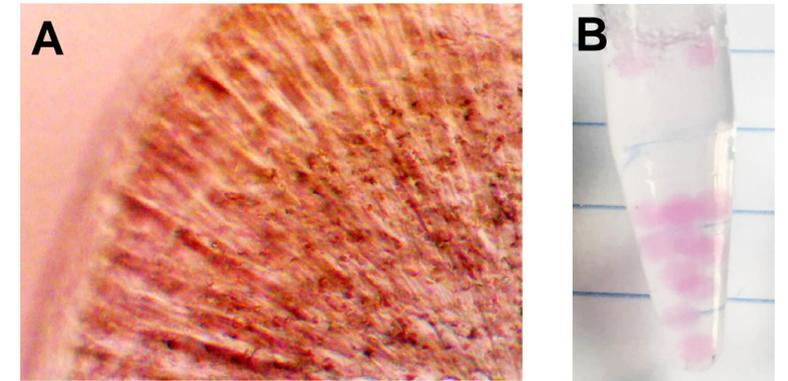
**Figure 3:** A) Microscope image of cell-seeded alginate bead at day 2 B) Eppendorf tube of cell-laden beads on day 2 before centrifugation and addition of sodium citrate
