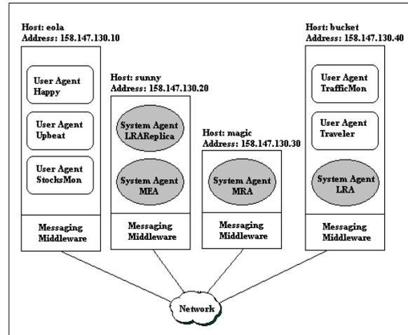
**Figure 2.3 – The AGI Architecture Hosts Configuration**
