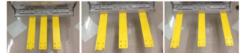
The forklift is capable of lifting up to 200 lbs. of dry weight. It was altered during our generation to include a mountable faceplate and adjustable fork width for a variety of operations. These alterations allow the operator to lift a range from smaller, delicate to larger, unwieldy artifacts off of the sea floor. The forklift, as well as, the other attachments, aid alongside divers for standalone applications.
