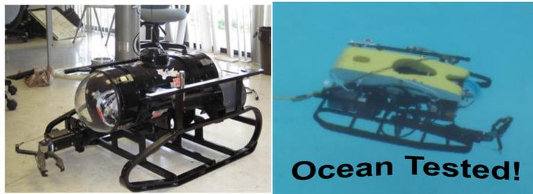
The body of the TOMCAT was sandblasted and repainted using an epoxy-based paint after a self-etching primer was applied. This new coat will keep the ROV from corrosive damage in long missions. Mounting plates were made for the thrusters to secure to the frame and reduce the risk of malfunction during deployment. The TOMCAT frame was also given I-bolts as lift points for easy deployment during a mission.
