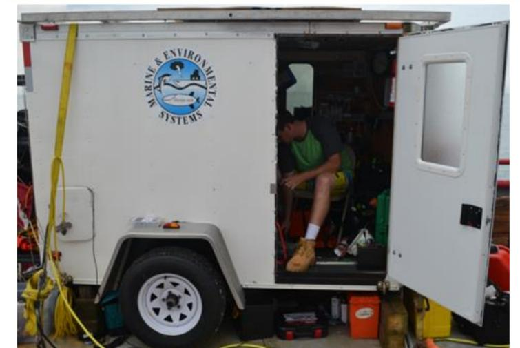
The purpose of the Mobile Command Center is to have a safe, comfortable and secluded area to operate the Crawler and TOMCAT. The command center was outfitted with windows, easy access door, air-conditioning, and worktable. This allows for versatility of the trailer and adaptation to any environment. The trailer is also equipped with lift points to be able to transfer it to any ship deck.
