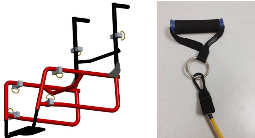
Clamps fixed to the wheelchair frame will allow for the attachment of resistance tubing of different lengths to accommodate a large range of core and shoulder exercises. Six levels of resistance tubing will be included with the device so the end user can select the strength of tubing that corresponds to his or her own upper body strength.
