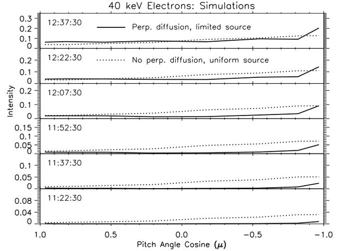
**Figure 3.** Simulation results for intensity as a function of  $\mu$  for different time in the 2001 September 24 event. The panels from bottom to the top show increasing time. Solid and dotted lines indicate simulation results at each time with and without perpendicular diffusion considered, respectively.
