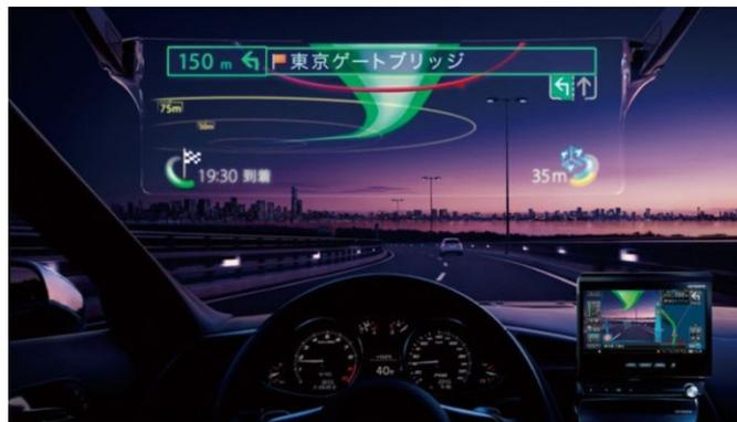
*Figure 2: Example of a Heads-Up Display.*
