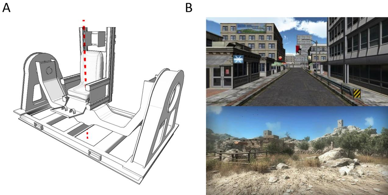
**Figure 1. MARS device and virtual environments used.** Left: MARS device. The yaw axis (red dashed line) was aligned with the gravitational vertical. The reference yaw orientation of  $0^\circ$  orients the chair facing forward, as shown. Positive angles in yaw rotate the chair clockwise. Right: Visual scenery used during training (top) and experiment (bottom). In both scenes, one unit in the virtual world equals one meter in the real world.
