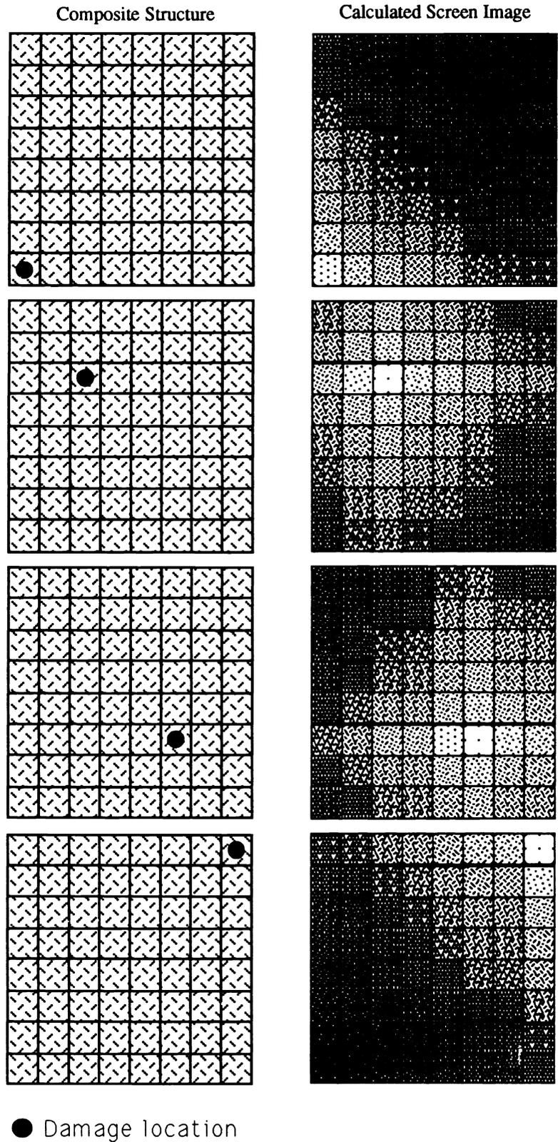
*Figure 9. Comparison of damage location and predicted image intensity distribution*
