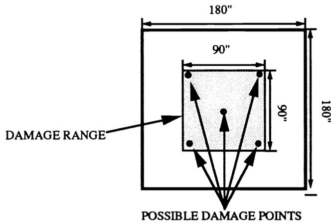
Figure 4. Composite plate and damage area
