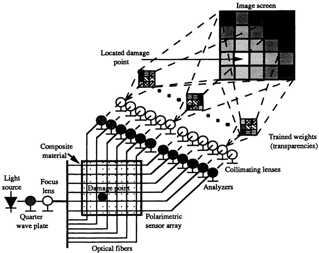
Figure 1. Schematic of all optical 2-D damage assessment system
