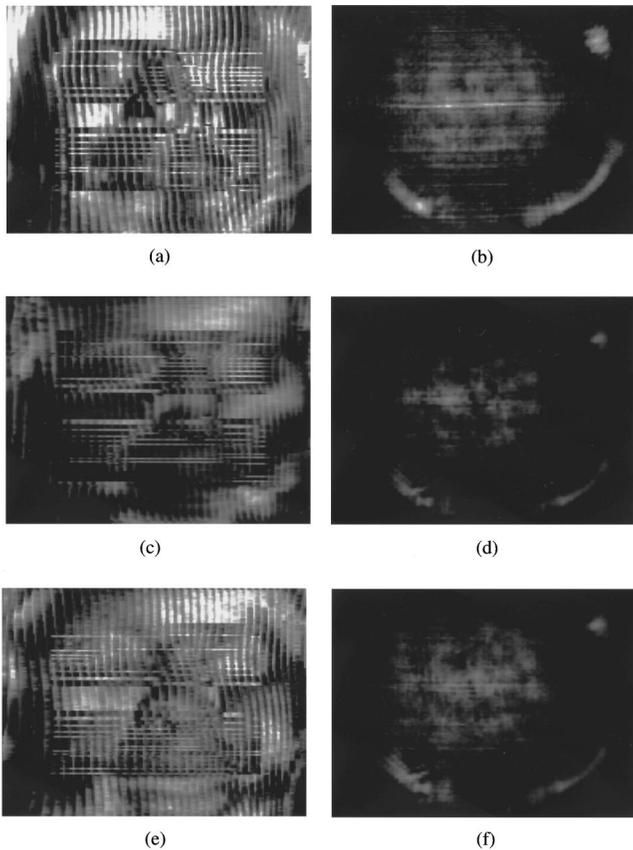
**Fig. 8** Results of face recognition experiment: (a) live mix as shown in Fig. 7, (b) output of the system indicating correct recognition, (c) live mix of filter grating with an incorrect face, (d) output of the system indicating no recognition, (e) live mix of filter grating with another incorrect face, and (f) output of the system indicating no recognition.
