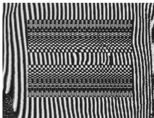
**Fig. 6** Filter grating obtained by combining the phase information in Fig. 5 and the cylindrical zone plate.
