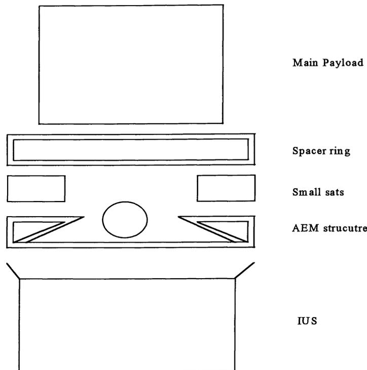
**Figure 1. Smallsat AEM bus and IUS stack**
