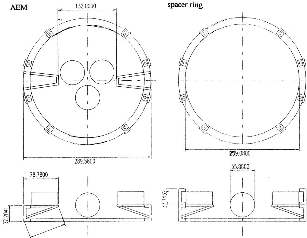
**Figure 2. Payload Support Structure (all dimensions are in centimeters)**
