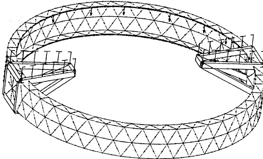
**Figure 3. Finite Element Model of the AEM truss structure**
