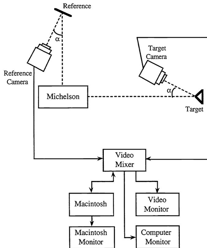
Figure 1 - Filter grating generating system
