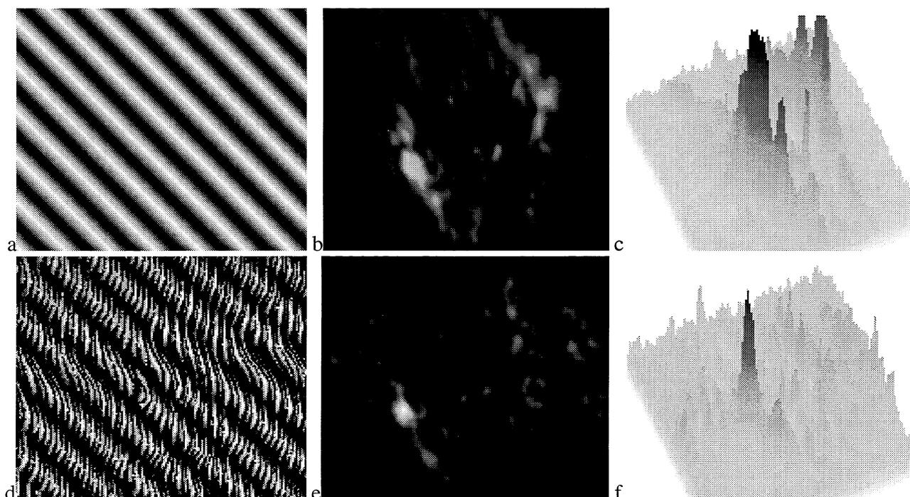
Figure 9 - a) Computer generated desired output, b) off axis components produced due to figure a, c) 3D plot of b, d) simulated desired output using XOR function, e) off axis component due to d, f) 3D plot of e.
