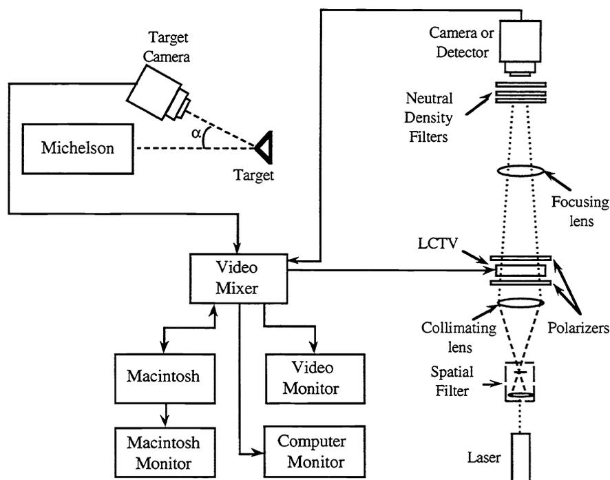
Figure 2 - Optical processor
