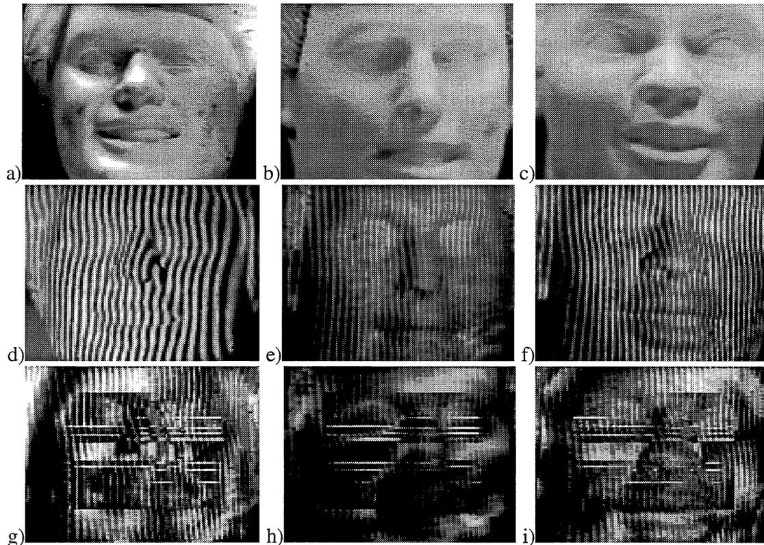
Figure 5 - a, b & c show the 3 targets under standard illumination; d, e & f correspond to the 3 targets under structured illumination; g, h & i are the outputs (live video mix) moiré patterns corresponding to the three faces.
