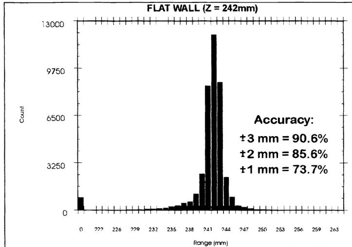
Fig. 3. Range histogram for a flat wall as measured by surface mapping system with 1:200 range resolution.
