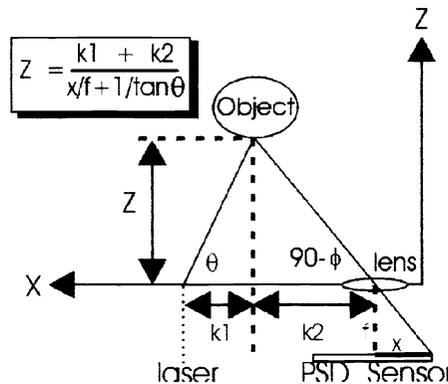
Fig. 2. Configuration of a flying spot laser scanner system used for underwater surface mapping.
