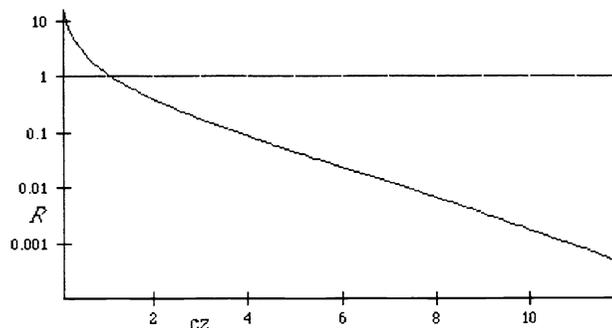
Fig. 1. The ratio  $R$  of  $E_d$  to  $E_s$  versus attenuation length  $cz$  for  $c/s = 3$ .
