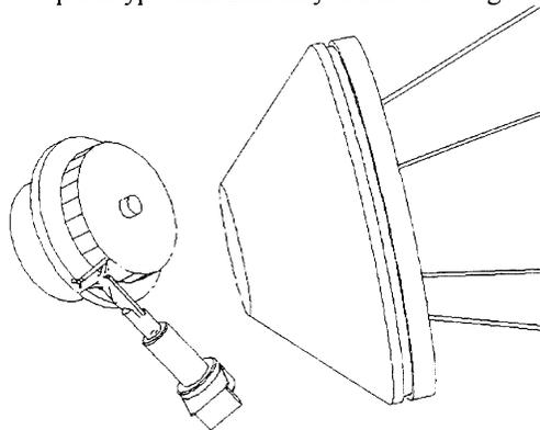
Fig. 7. Scanner design used in the prototype geological profiling system, showing optical pressure port (rightmost), rotating horizontal scan mirror (upper) and vertical scan galvanometer (lower). Laser scan limits are shown exiting the window.
