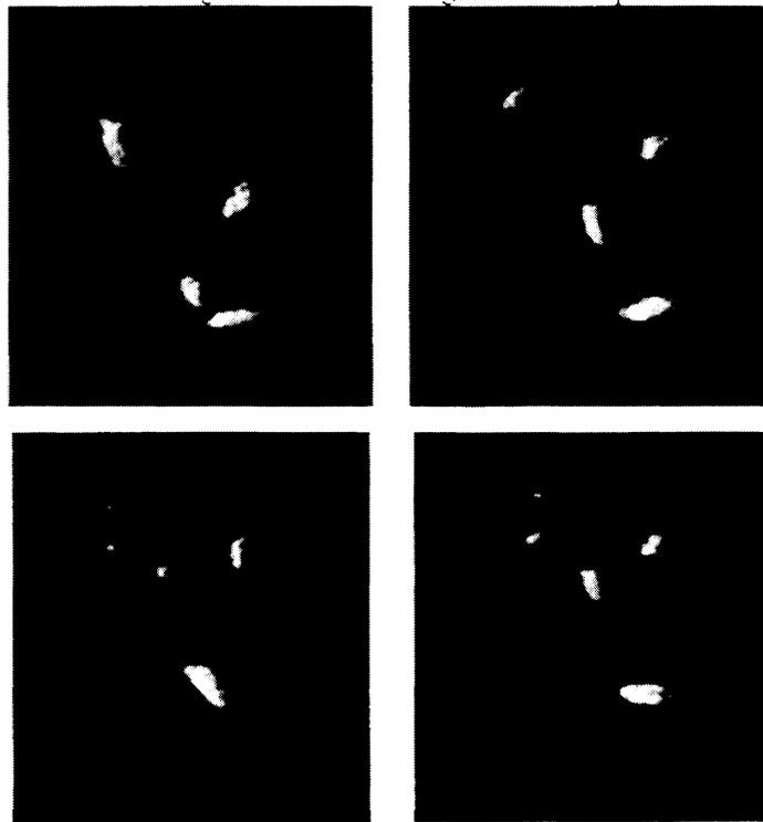
Fig. 5. 3-D pseudo-color range image of fish swimming in clear water taken at an acquisition rate of 20/second.
