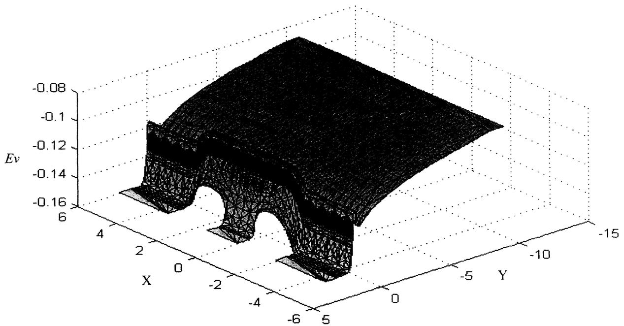
Figure 3 Valence band diagram shown in 3-D
