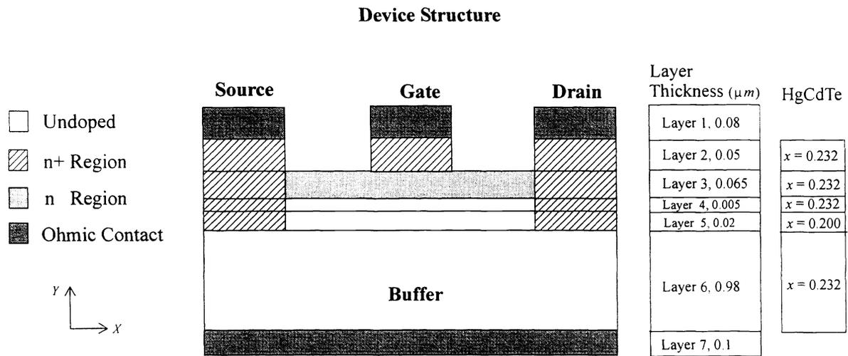
Figure 2 Schematic cross section of the HgCdTe PHEMT
