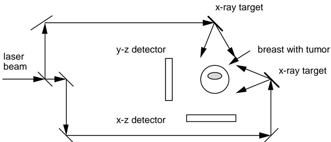
Figure 2. Arrangement of x-ray sources to enable three-dimensional location of tumor and guidance of biopsy needle.
