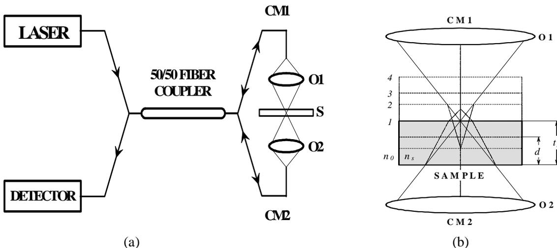
Figure 5. Experimental optical setup (a) and operating principle (b) of a dual-confocal fiber-optic sensor. Laser, He-Ne laser (632.8 nm); 50/50 Fiber Coupler, a 2×2 50/50 (3 dB) OF coupler; O1, O2, confocal focusing objectives; CM1, CM2, the first and second confocal microscope; Detector, a precise digital powermeter;  $d$ , sample displacement;  $t_s$ , sample thickness;  $n_0$ , refractive-index of the surrounding area;  $n_s$ , sample refractive-index.
