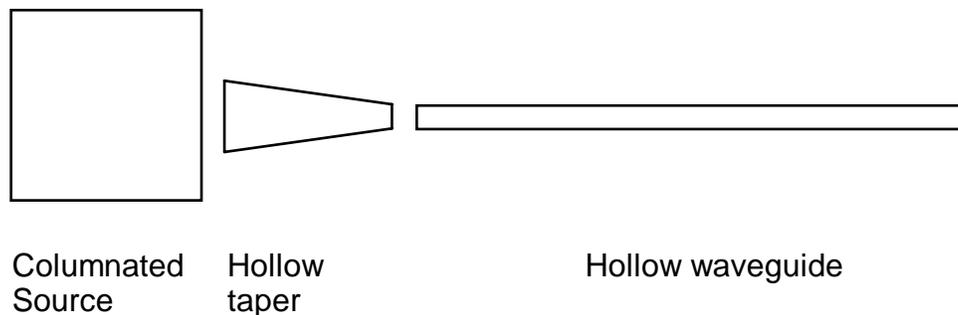
Figure 3. Delivery system for terahertz to x-ray radiation.
