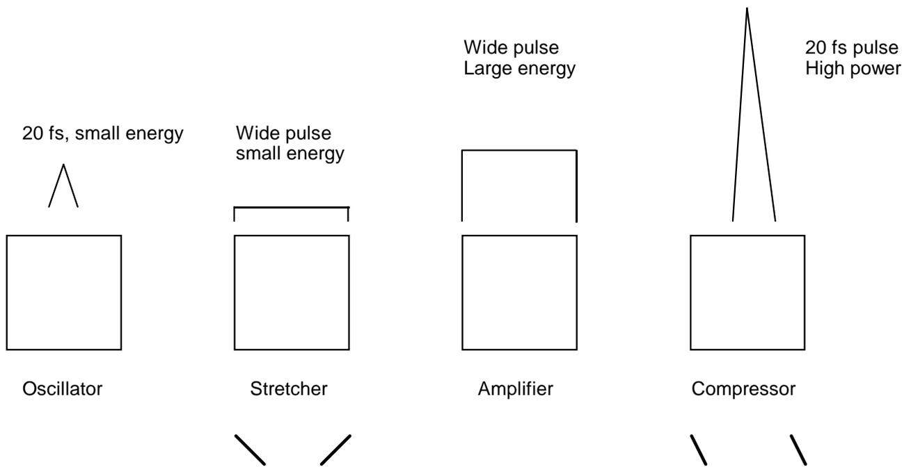
Figure 1. Diagram of Ti:sapphire chirped pulse amplification for high power laser beam to produce hard x-ray emission. [After ref # 2.]
