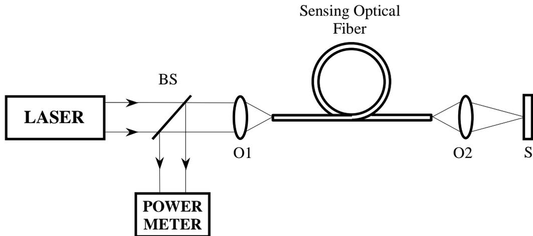
Figure 4. Fiber-Optic Confocal Microscope. Laser, He-Ne laser (632.8 nm); BS, beam-splitter cube; O1, O2, microscope objectives..
