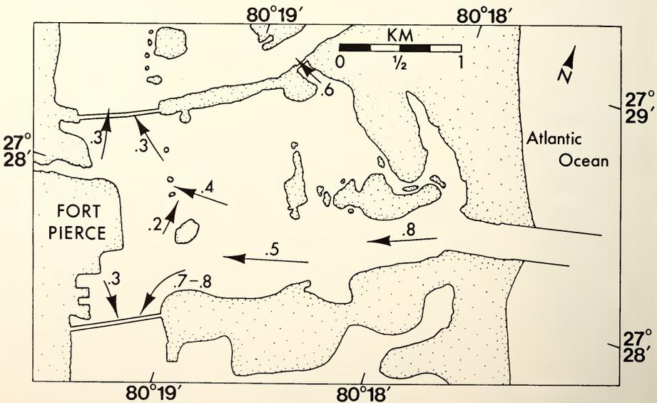
FIG. 5. Subsurface flood current pattern.
