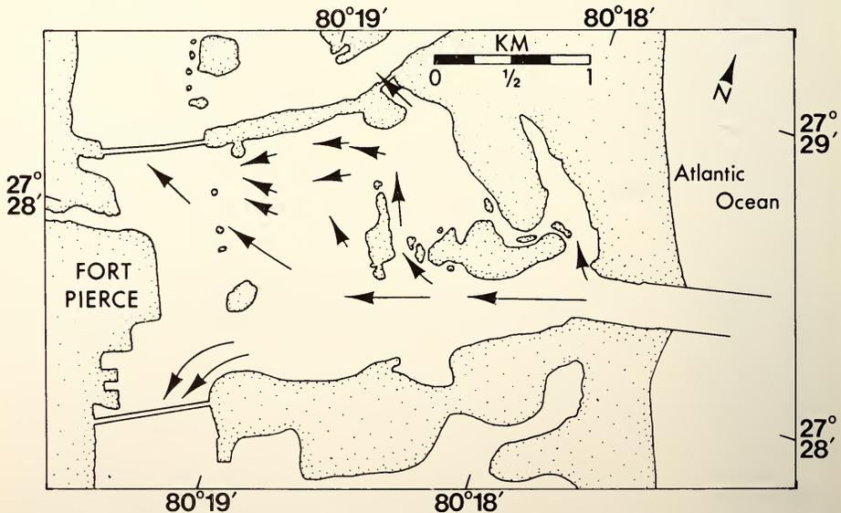
FIG. 2. Surface flood current pattern.
