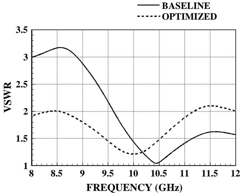
Fig. 5. VSWR versus frequency for baseline and optimized geometries
