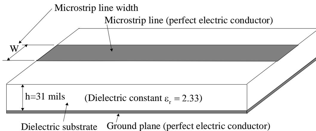
Fig. 3. Microstrip line geometry
