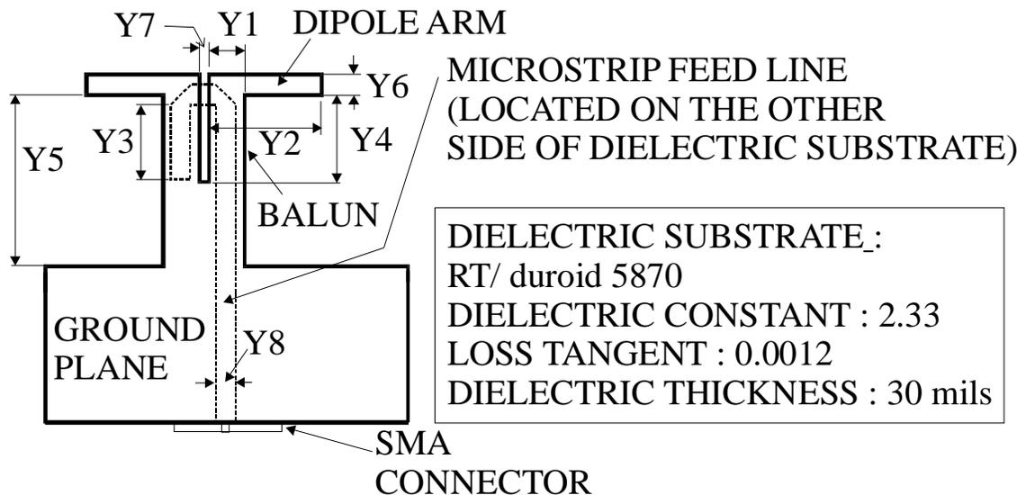
Fig. 4. Diagram showing geometry of the printed dipole structure and geometrical parameters Y1 to Y8
