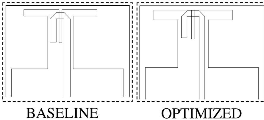
Fig. 6. Scaled geometry corresponding to baseline and optimized cases
