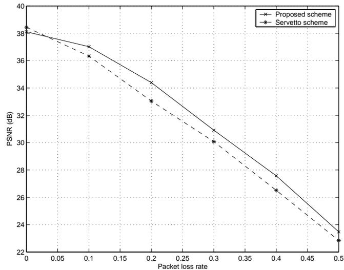
**Figure 5:** Reconstruction quality vs. packet loss rate
