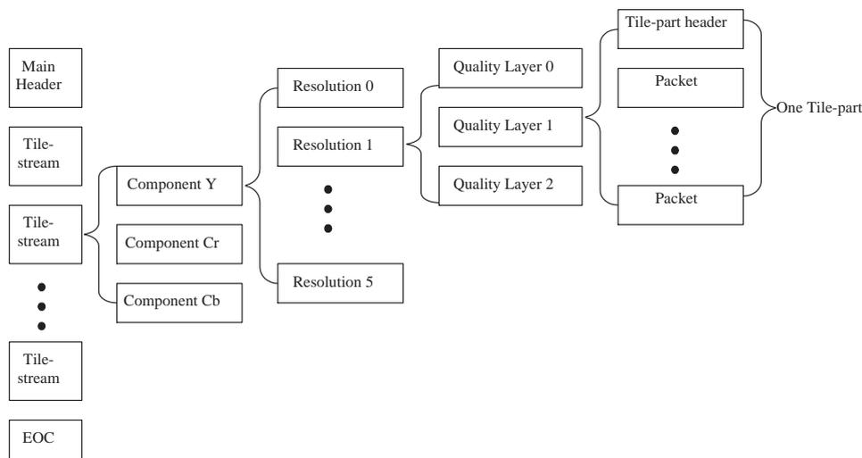
Figure 3. The structure of of a JPEG-2000 bitstream.
