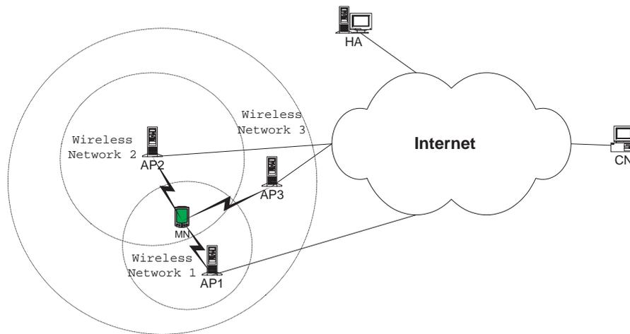
**Figure 4.** Mobile IP/IPv6 and wireless overlay networks.
