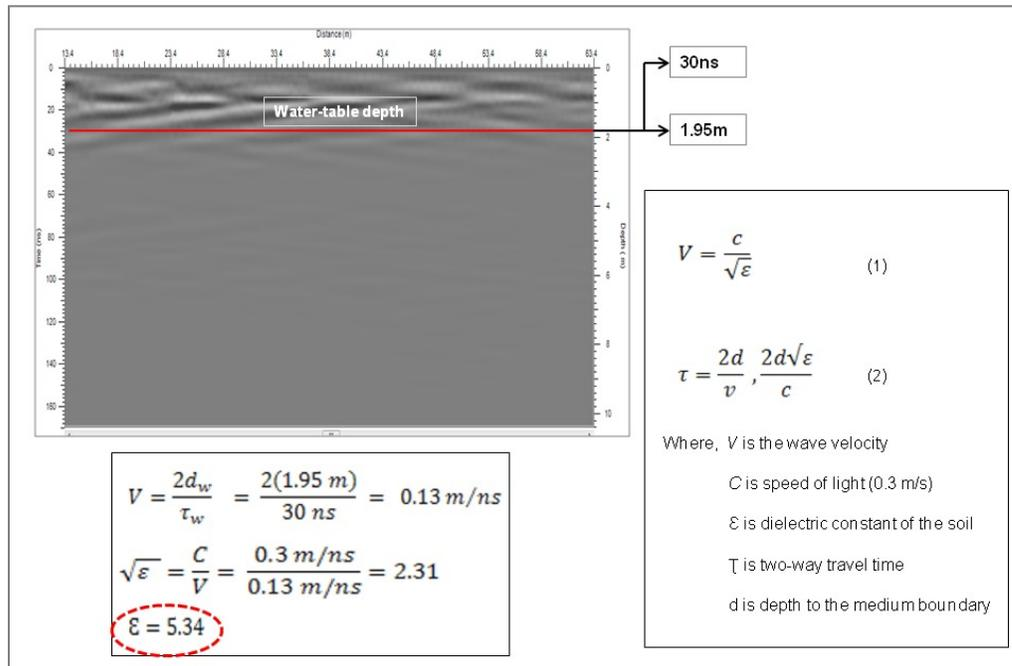
Figure 11. GPR profile showing location of the water table depth and equations used to determine velocity, two-way travel time and dielectric constants.
