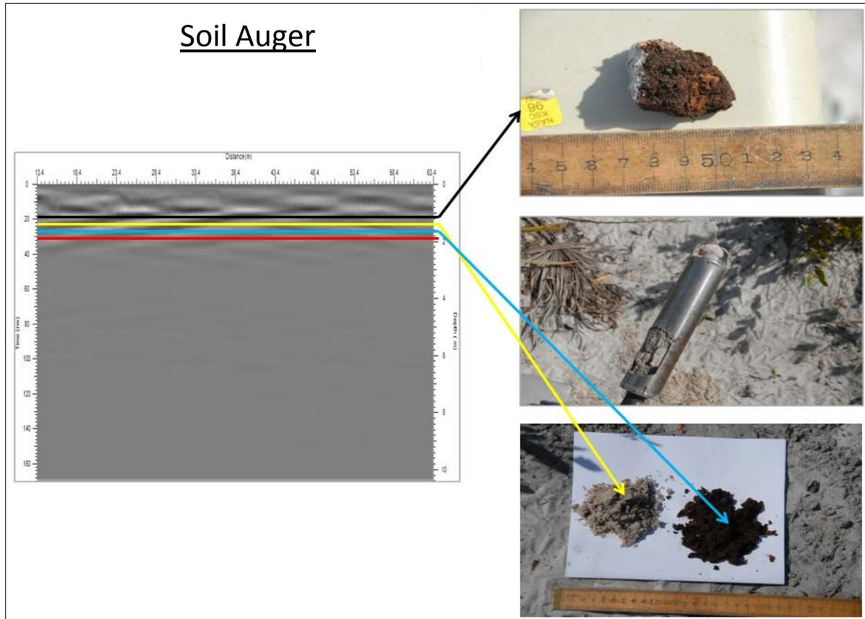
Figure 10. Water table depth and different soils as estimated by the soil auger.
