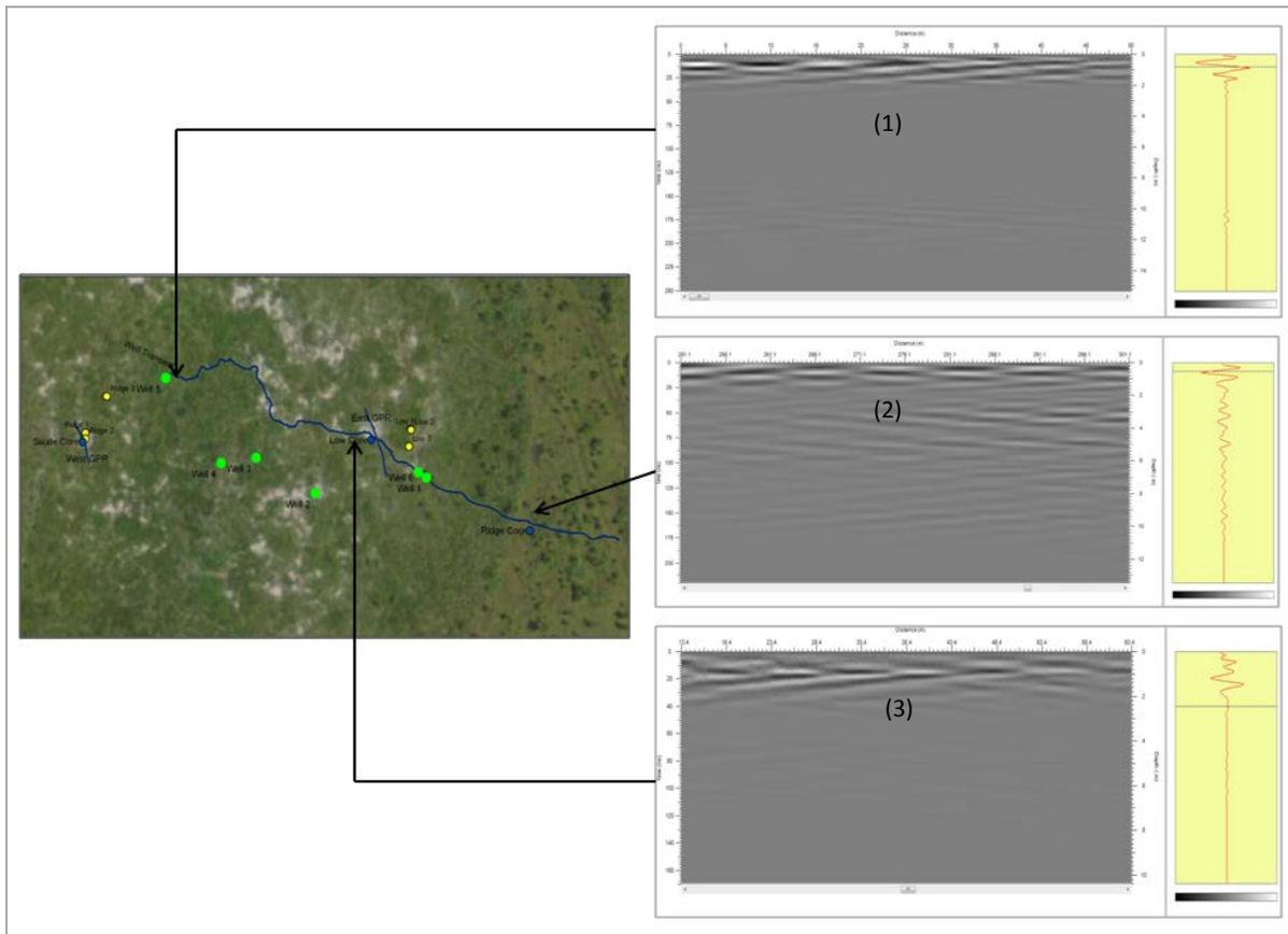
Figure 5. GPR profiles and trace window from different elevations along the GPR transect.
