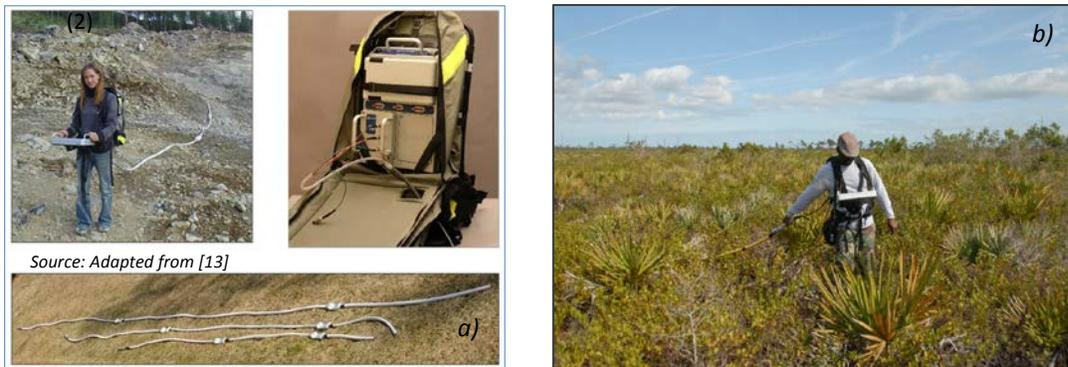
Figure 1. GPR system (ProEx unit and the RTA antenna).
