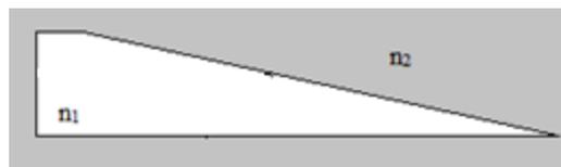
Figure 5: Bevel edged fiber with  $n_1$  being the index of the core material while  $n_2$  is free space.
