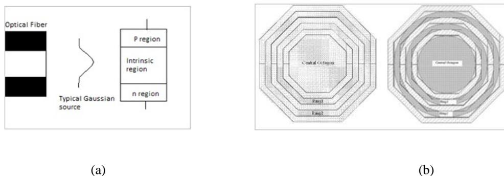
Figure 3: (a) Typical Gaussian profile from an optical fiber impinges upon a PIN diode to generate photo-current. (b) Concentric three channel CMOS photodiode structure is shown on the left while the picture on right shows the CMOS design with a typical SDM incident upon the diode.
