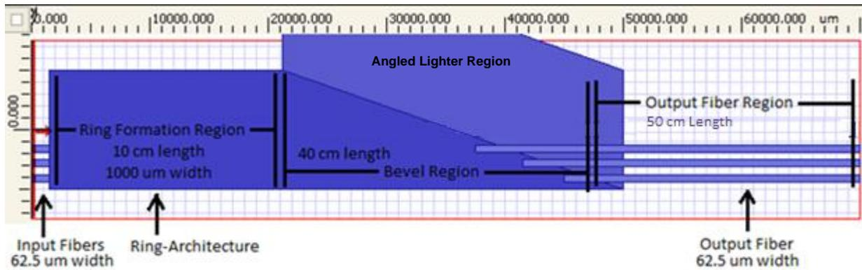
Figure 7: OptiBPM design showing the three key regions (not to scale). The darker region in the first half of the figure shows the hollow core fibers with the input fibers to the left of it. The angled lighter region indicates cladding with refractive index of 1 and the output fibers are to the right of it.
