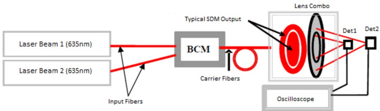
Figure 1: Block diagram of the Beam Combiner Module (BCM) or the multiplexer of the SDM system.
