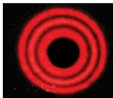
Figure 2: Output beam profile for a three channel SDM system.
