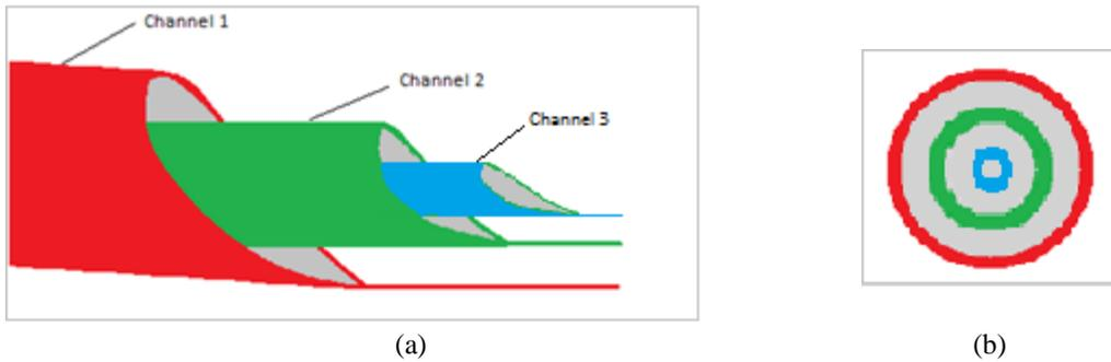
Figure 4: Core architecture for SDM output for three channels. This figure shows the general layout of the design with figure ‘a’ showing three dimensional side view of the presented architecture while figure ‘b’ shows two dimensional the top view.
