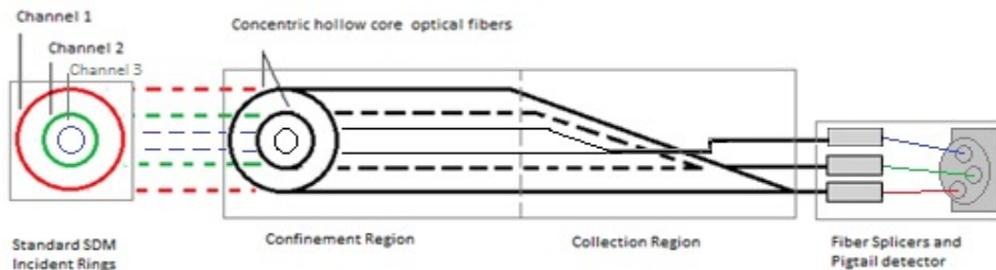
Figure 6: Architecture of the all optical De-Multiplexer. Data channels from carrier fiber are coupled into an array of concentric hollow core fibers that tapers down to guide optical energy into independent fibers or pigtail photo-detectors.
