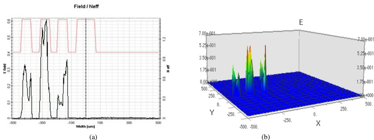
Figure 9: (a) Normalized E-field intensities confined within the core regions of the three fibers. The core region of the 4<sup>th</sup> fiber that is located at the origin is not illuminated.
