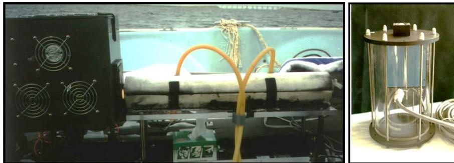
Figure 4. Shipboard long pathlength cuvette used to collect *in-situ* absorption spectrums (left) from continuously pumped water. *In-situ* submersible spectrograph (right) for collecting bottom reflectance signatures (BRF's) of bottom types used in equation 6.
