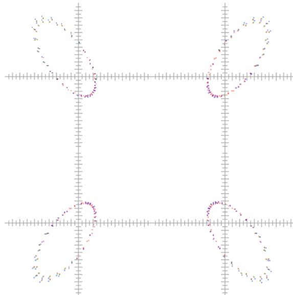
Figure 4: Results from OSLO simulation. All angles presented are for 45 degrees; however with different rotations of the x and y axes. Top-left: counter clockwise (CCW)-X, CCW-Y. Top-Right: CCW-X, Clockwise (CW)-Y. Bottom-Left: CW-X, CCW-Y. Bottom-Right: CW-X, CW-Y. Note that this image is on a slightly different scale than figure 3.
