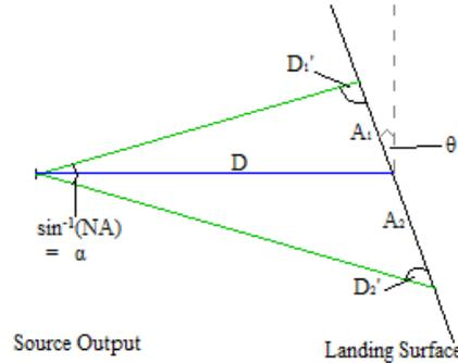
Figure 7: Theoretical model of the output of the proposed device. The rings leaving the device will spread as a function of the fiber's numerical aperture. The  $\theta$  term is the incline of the landing surface.
