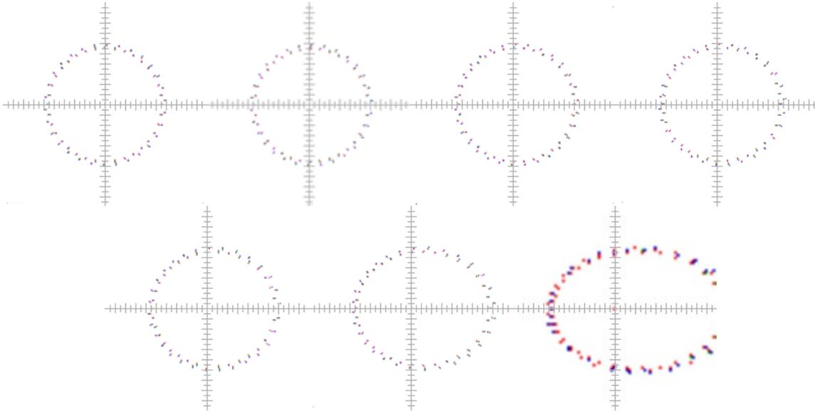
Figure 3: Simulated ring pattern using the spot diagram function in OSLO. The ring pattern is displayed by rotating the image surface in the clockwise direction. The patterns results for following angles are presented from top left to bottom right:  $0^{\circ}$ ,  $5^{\circ}$ ,  $10^{\circ}$ ,  $15^{\circ}$ ,  $20^{\circ}$ ,  $30^{\circ}$ , and  $45^{\circ}$ . The central dot for all patterns is located at the vertices of the axes.
