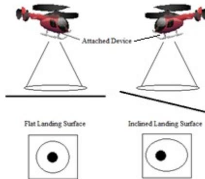
Figure 1: Graphic representation of the proposed landing aid. On a flat surface when the VTOL is aligned, the output signal appears exactly the same as an input signal; however, in case of an inclined surface or unaligned VTOL, the output will assume an elliptical shape with unequal distances between the central spot and complementary edges of the projected circle.
