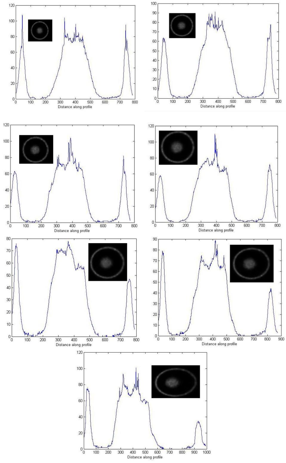
Figure 6: Intensity profiles for experimental data. Angles of rotation are as follows starting from top left to the bottom graph: 0°, 5°, 10°, 15°, 20°, 30°, and 45°.
