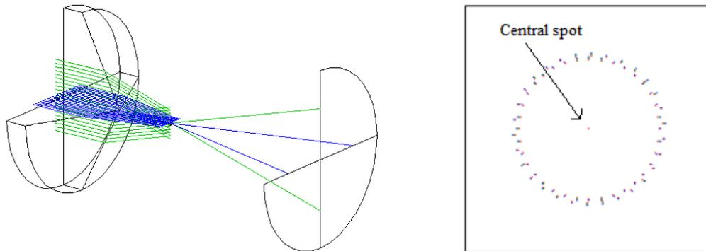
Figure 2: An axicon lens simulates the desired optical pattern. A small aperture limits generated rings to two. The image on the left shows the lens setup while that on the right shows spot diagram for zero degree rotated image plane, simulating a flat landing surface.
