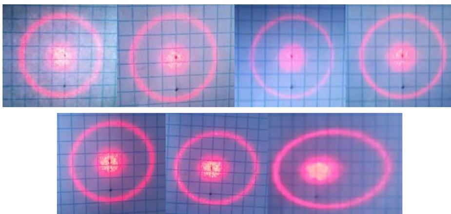
Figure 5: Experimental data using SDM method of generating rings. The screen is rotated in a clockwise direction. The angles are as follows going from the top left image to the bottom right image:  $0^{\circ}$ ,  $5^{\circ}$ ,  $10^{\circ}$ ,  $15^{\circ}$ ,  $20^{\circ}$ ,  $30^{\circ}$ , and  $45^{\circ}$ .
