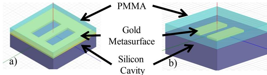
Figure 2. a) A unit cell of a FRMM consists of a dual nanoslotmetasurface of ellipsometric measured<sup>20</sup> gold optical properties on top of a silicon cavity. The resonant coupling structure consisted of a PMMA overlay on top of the FRMM. b) Similarly, the complementary unit cell FRMM metasurface (dual nanorod) is shown.
