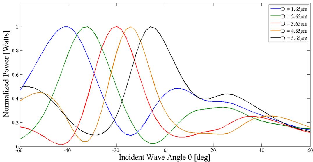
Figure 3: Normalized power dissipated in Ni bolometer versus incident wave angle for different distances  $D$  of bolometer, from the LWA, on the transmission line.
