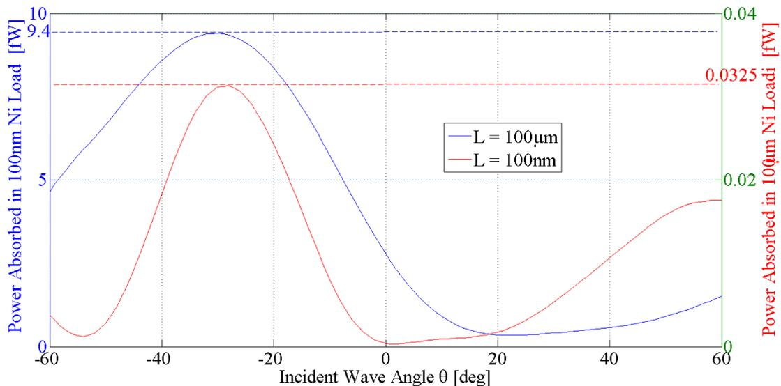
Figure 5: Improvement in power absorbed in Ni load through extension of load length.
