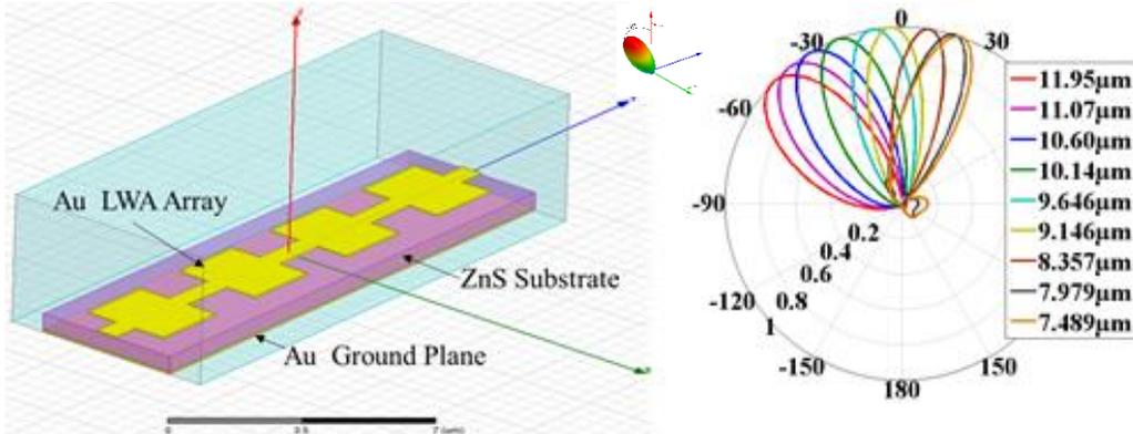
Figure 1: IR leaky-wave antenna array (a) geometry (b) frequency scanning behavior with  $\theta = -30^\circ$  beam at  $10.6\mu\text{m}$  in the YZ ( $\varphi = 90^\circ$ ) plane.
