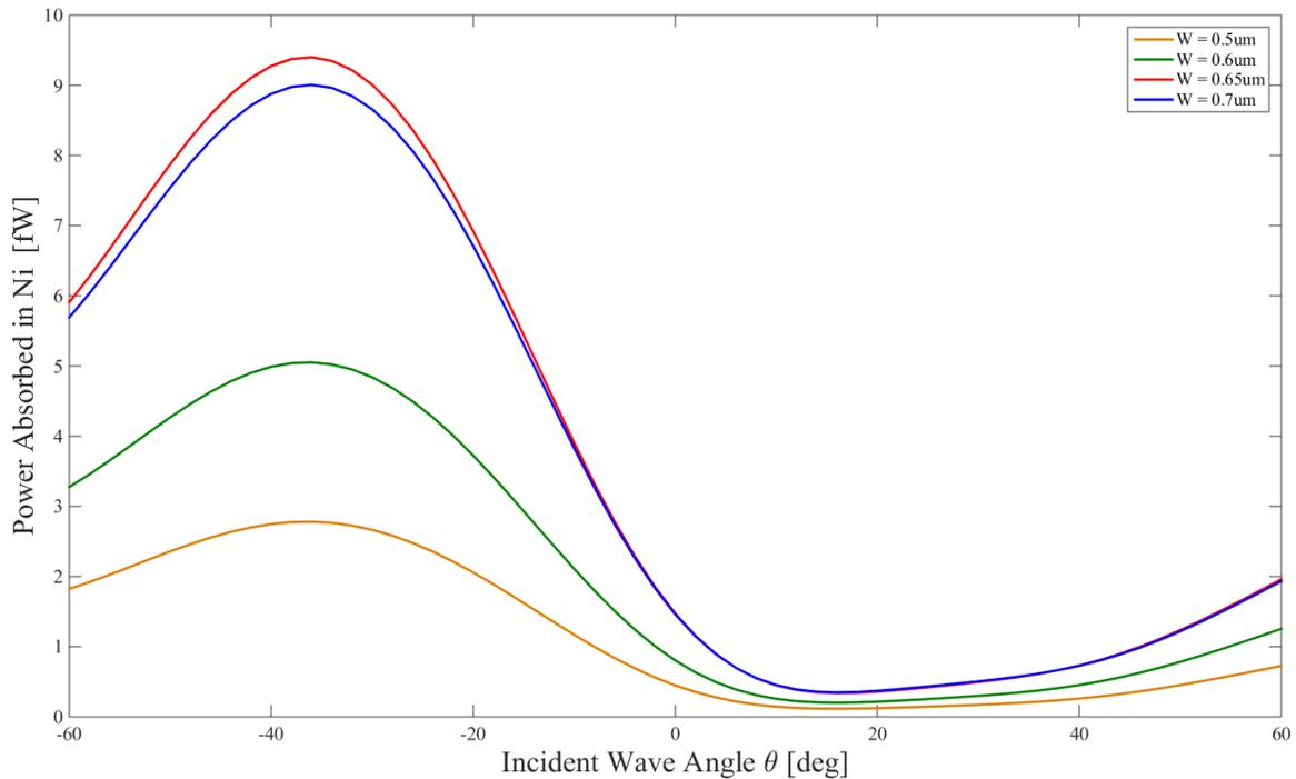
Figure 6: Variation in power absorbed in Ni load for different widths of transmission line type load.
