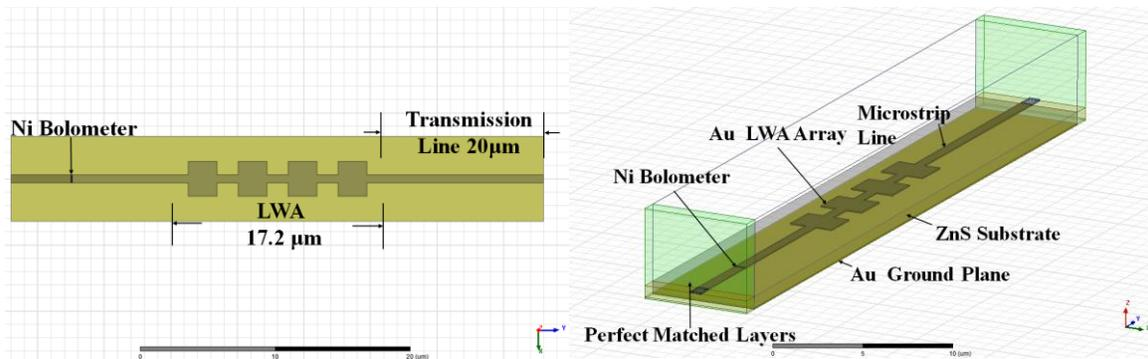
Figure 2: Geometry of IR LWA loaded with Ni bolometer.
