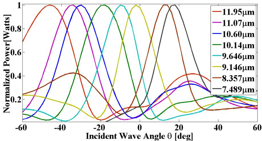
Figure 4: Frequency scanning behavior of the signal collected in the bolometer with  $-30^\circ$  at  $10.6\mu\text{m}$  and near broad side at  $9.15\mu\text{m}$  for a bolometer placed  $2.65\mu\text{m}$  away from the LWA.
