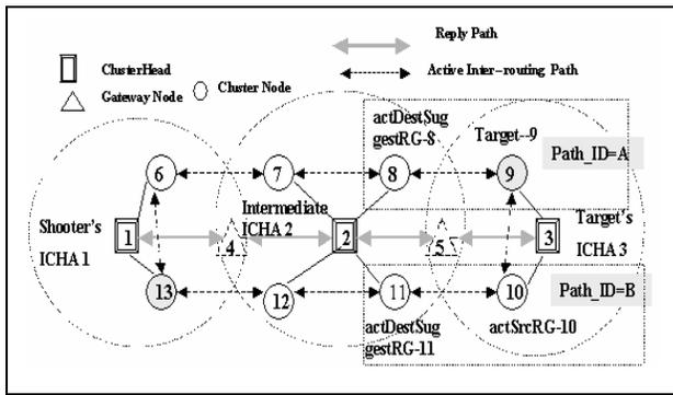
Figure 8: Target's ICHA-3 received RREQ and determined multi inter routing path
