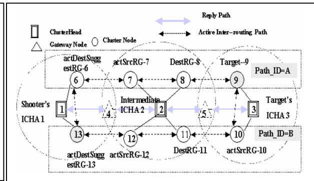
Figure 9: Intermediate's ICHA-2 received RREQ message and determined multi inter routing path.
