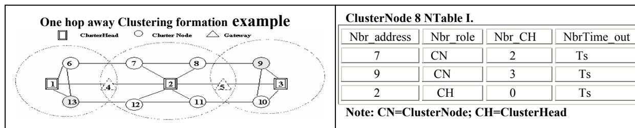
Figure 1: illustration one-hop away Clustering formation and Neighbor Table maintaining example.
