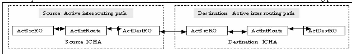
Figure 13: Illustration the two active inter routing path are connected by route gateway (actDestRG and actSrcRG).
