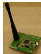
Figure 2: Chipcon CC1010EM with Antenna
