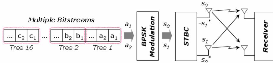
Figure 4: Procedure from multiple bitstreams to STBC.
