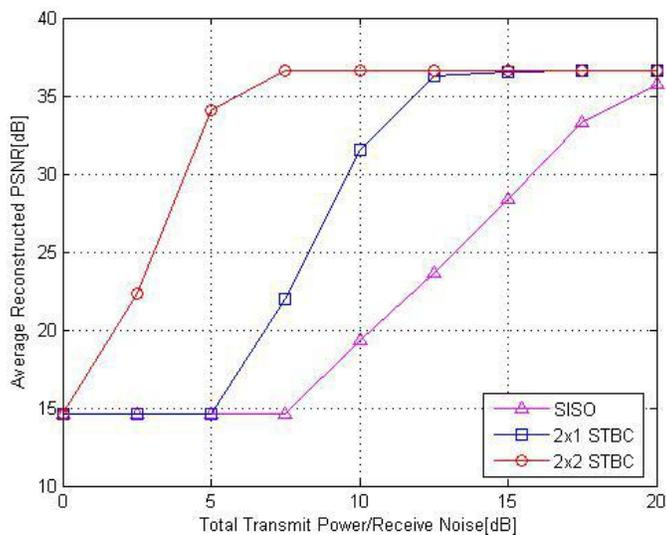
Figure 6: PSNR gain of MIMO wireless systems in Rayleigh flat fading channel.
