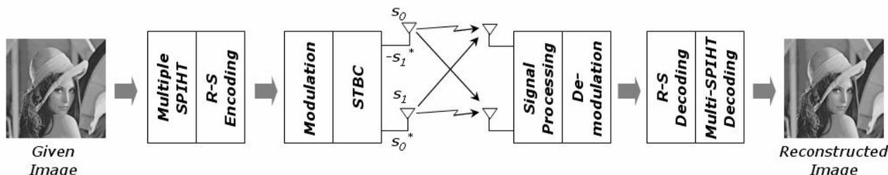
Figure 1: Illustration of the proposed robust image transmission system.
