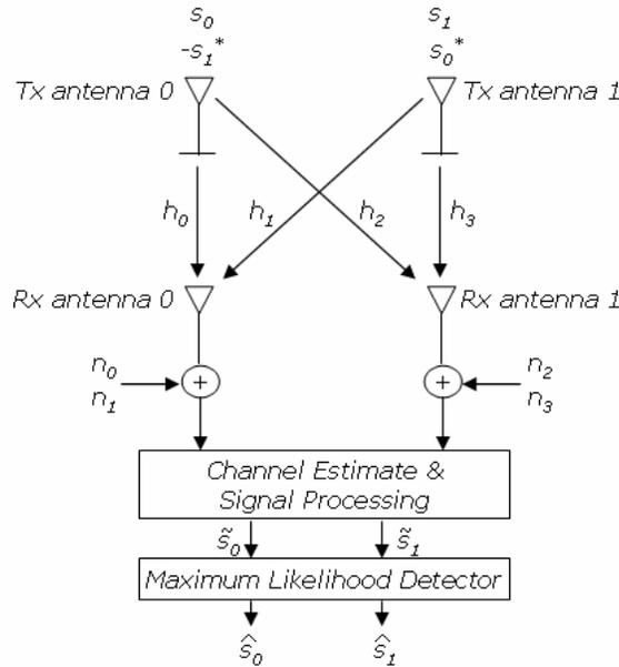
Figure 3: MIMO system with two transmit and receiver antennas.
