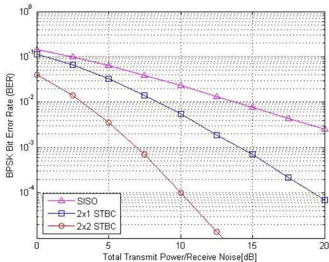
Figure 5: BER performance of coherent BPSK in Rayleigh flat fading channel.
