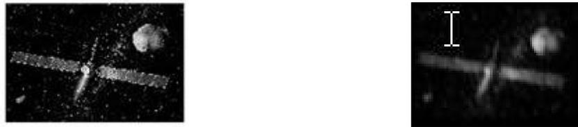
**Figure 2: Left is the un-aberrated reference object brightness. Right is the aberrated image generated using the 4<sup>th</sup> through 6<sup>th</sup> Zernike polynomials all weighted by 2 radians.**
