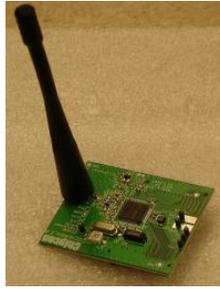
Figure 4: Chipcon CC1010EM with Antenna
