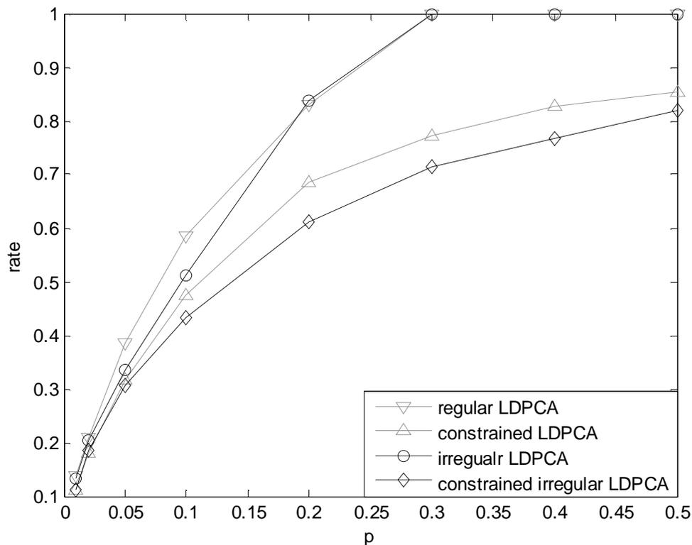
Figure 3 Performance of constrained LDPC decoder comparing with conventional SPA
