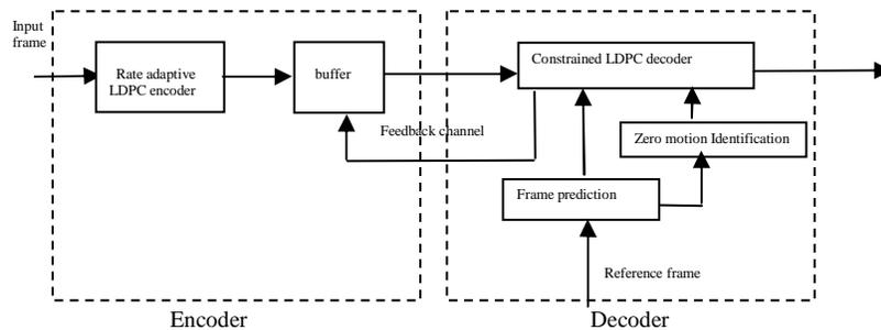
Figure. 1 Architecture of proposed distributed video source codec
