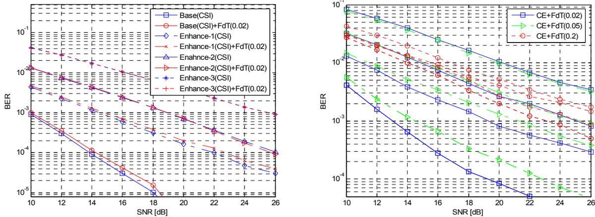
Figure 5: BER performance of ACS-MIMO system (left) BER against feedback delay (right) BER against CE error and feedback delay
