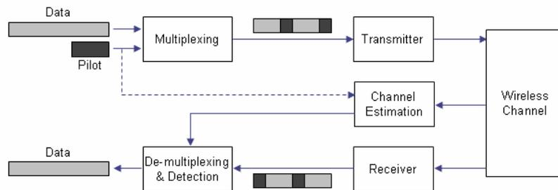
Figure 3: Block diagram of a PAT transceiver
