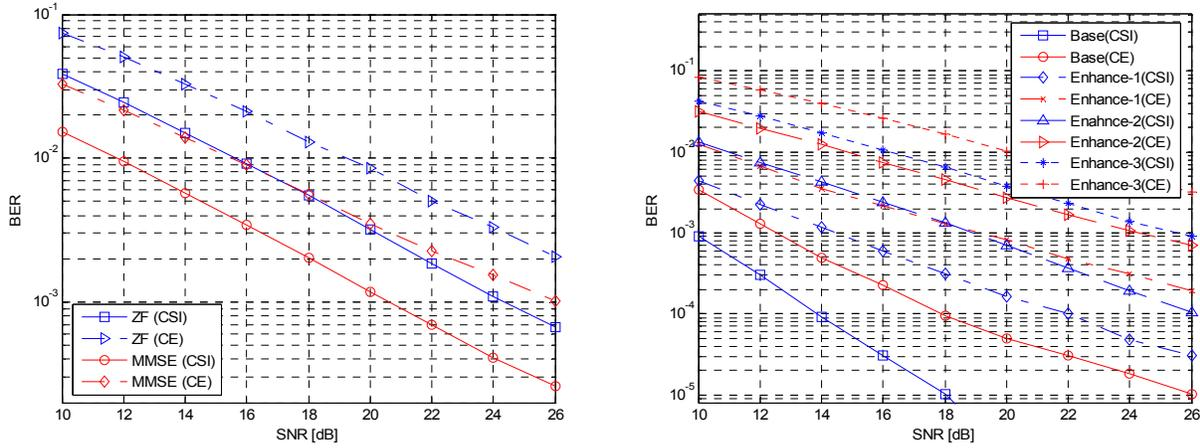
Figure 4: BER performance of ACS-MIMO vs. OL-MIMO (left) OL-MIMO system without ACS (right) proposed ACS-MIMO system
