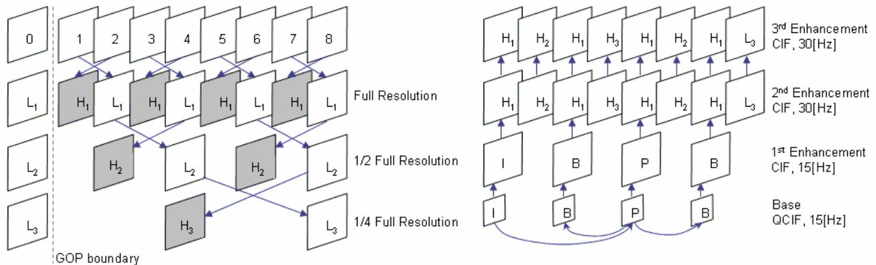
Figure 2: Scalable extension of H.264/AVC scalability
