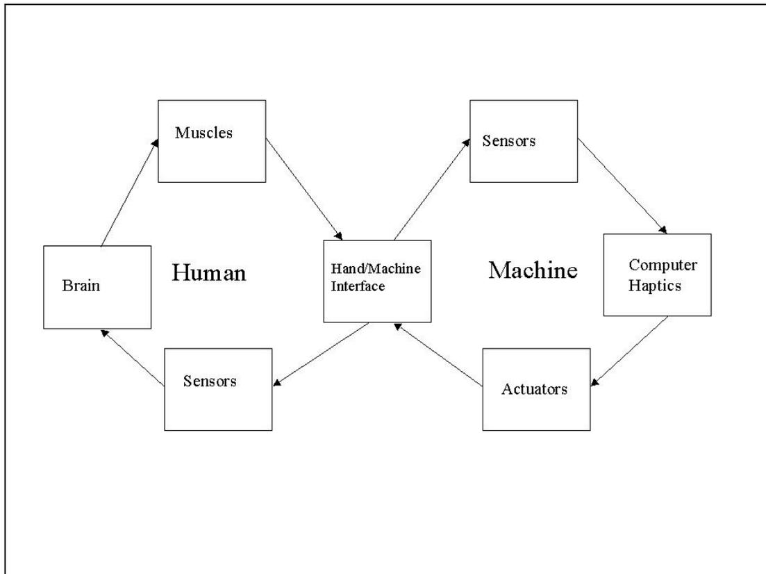
**Figure 4.** Haptic interaction between human and machine. (From Srinivasan, 1997)
